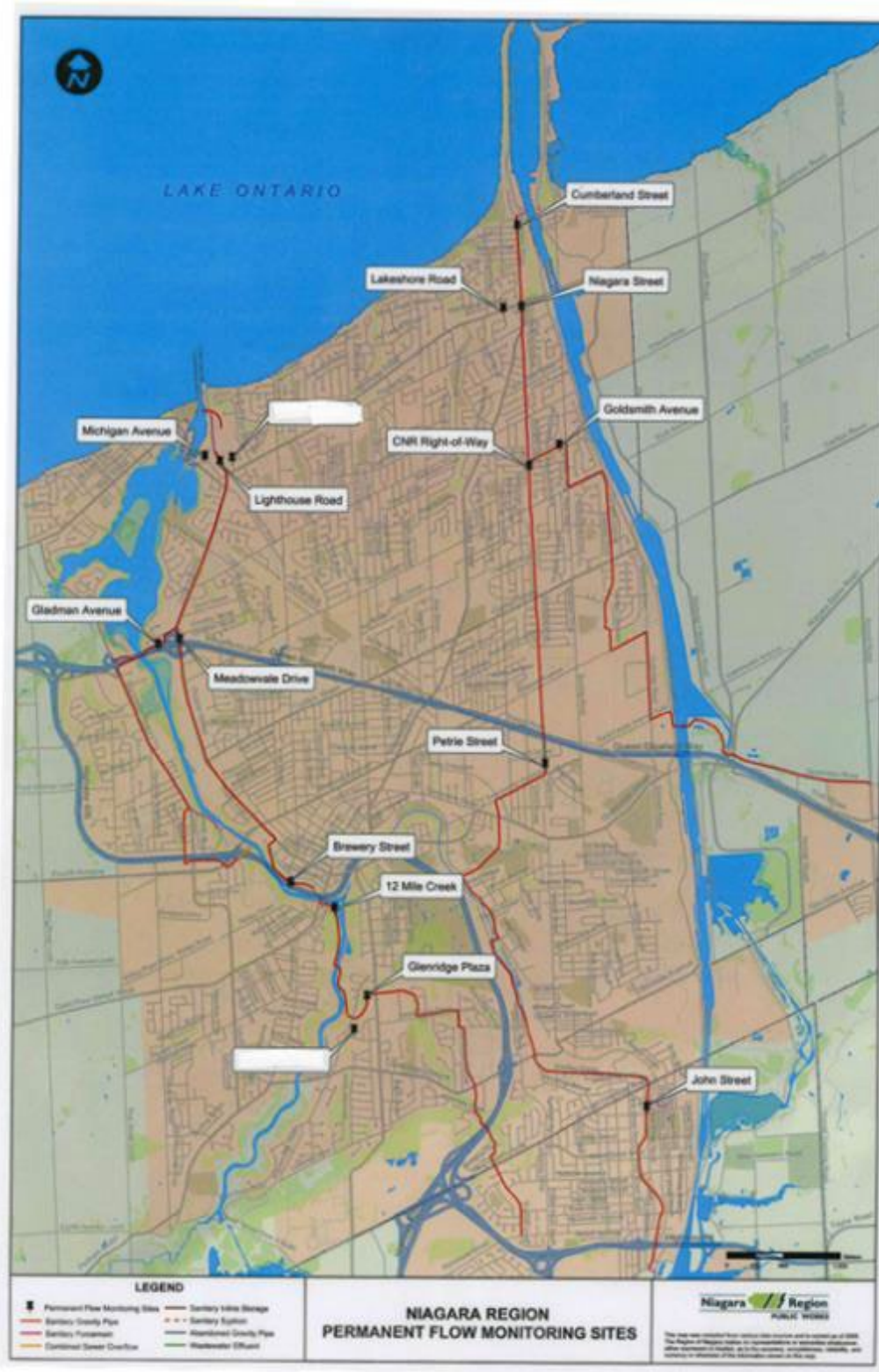
Figure 6-2: Permanent Sewer Flow Meters Operated by the Region of Niagara
